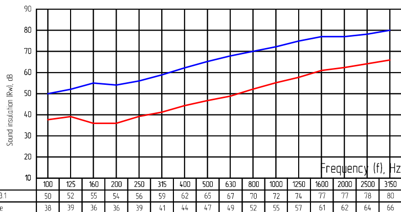
Airborne noise insulation frequency response, R_w(f)
